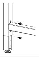
Align Frame of assembled Unit B (Frame & Leg only) with threaded inserts located on front of Frame on Unit A (upright and assembly) using KIT-05A. Tighten hardware.
