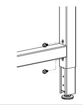
Position Frames flush to rear edge of Worksurface. Position Swaybrace on Frame followed by Legs. Fasten Swaybraces to back of Legs using KIT-21. Where Swaybraces abut at Intermediate Leg, install Joining Plate with KIT-23A.
