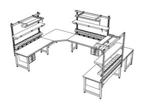
A U-shape configuration makes the most of limited square footage for a test and repair application. Three identical work set-ups were provided with adjustable overtable accessories including powerstrips, mounting rails with plastic bins, shelves, and light suspension systems. A hanging drawer case at each station stores small parks and hand tools. The two corner sections provide a buffer zone between stations and additional work surface or storage space for shared access.
