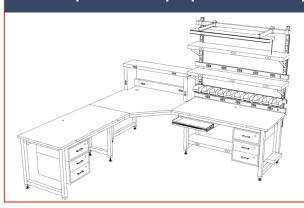
A length of nine feet in each direction provided a much needed work surface for a repair operation. Overhead storage, lighting and power accessories are concentrated on one wing for intensive repair functions, while the remaining wing is kept open.
