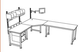
An 8'x10x30"D work space was specified for the repair and inspection of high vacuum valves. The Series 5300 unit is equipped with accessories including hanging drawers, a 20-amp wiretrough, adjustable divider shelf, and articulating monitor arm.
