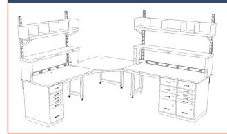
A 9'x10'x36"H workstation features three cabinet supports to accommodate the volume of drawer storage space required. Fixed riser shelves and adjustable overtable divider shelves provide additional equipment storage. Power needs are met with two 15-amp powerstrips.
