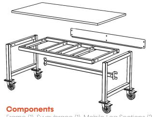
Frame (1), Swaybrace (1), Mobile Leg Sections (2), Casters (4), Swaybar (1), Worksurface (1)
