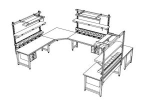
A U-shape configuration makes the most of limited square footage for a test and repair application. Three identical work set-ups were provided with adjustable overtable accessories including powerstrips, mounting rails with plastic bins, shelves, and light supsentions systems. A hanging drawer case at each station stores small parks and hand tools. The two corner sections provide a buffer zone between stations and additional work surface or storage space for shared access.
