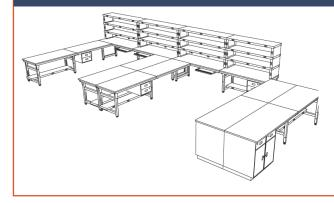
Triple-tiered fixed riser assemblies play a major role in the configuration of this work area, providing the space to house a myriad of equipment. In-line rows of Series 1000 tables are joined to the back row of tables, and are used back-to-back, making the most efficient use of valuable floor space.
