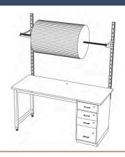
A Series 7200 Cabinet-to-Leg Technician Station is configured with a conductive top, Double Standard Uprights, and a Bubble-Wrap Mounting System which was designed and manufactured to meet this particular computer component manufacturer's requirement.
