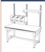
Simple, but efficient. Series 4500 unit with overtable divider shelf, adjustable to any height along the vertical double standard uprights.
