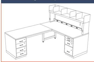
An L-shape corner unit was designed to fulfill a requirement for returns processing. Cabinets provide needed storage space; 15-amp Power Strip delivers power; and Fixed Riser Shelf with Divider System handles documentation materials. This particular unit was specified as a 30"Dx72"L station with a 30"x60" wing, although several sizes are available.
