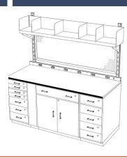
Series 7000 components designed the base of this unit. 2 single cabinets, one double cabinet, along with filler piece make up the 30"x72"Lx36H. Overtable accessories include powerstrip, pegboard, divider shelf on double standard uprights.
