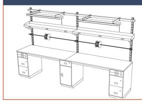
A Series 7000 Technician Station in-line row was selected for this shipping and receiving application. The row's dimensions are 30"Dx144"L with a 36" work height. Overtable accessories specified are spool holders, adjustable overtable shelves with back and end stops, and light suspension systems. Identical multi-drawer cabinets flank each end of the row, while a cabinet with a hinged door (with adjustable inside shelf) is centrally located.
