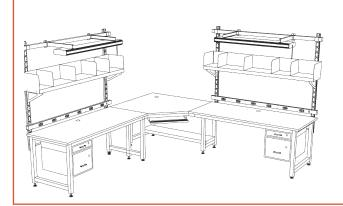
A Series 5300 Quad work center serves the needs of this verification center. Station is equipped with drawer storage, powerstrips, divider shelves, and undertable shelf, keyboard tray, and light suspension systems.
