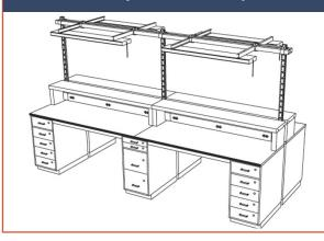
This four-person assembly station was configured with two Series 7000 Technician Station in-line rows, positioned backto-back. Fixed riser shelf assemblies, 20-amp wiretroughs, and light suspension systems complete the station.
