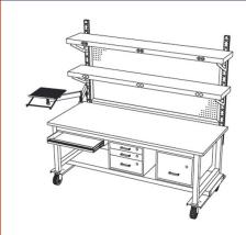
Another version of a mobile assembly unit, this Series 4500 mobile table is equipped with all of the features needed to aid in the assembly process. Note that overtable shelves may be specified with or without 20-amp duplex outlets to provide needed overtable power.
