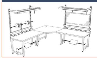
A Series 5300 Quad work center was selected for this assembly application. With dimensions of 9'  $\times$  9', the unit includes a variety of add-on accessories selected with specific work tasks and operator comfort in mind.
