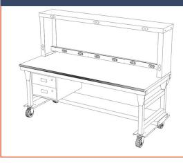
A mobile R&D workstation was designed with the Series 1000 Mobile Table, topped with a post-framed plastic laminate worksurface. Hanging drawers, powerstrip, and fixed riser shelf assembly complete this unit.
