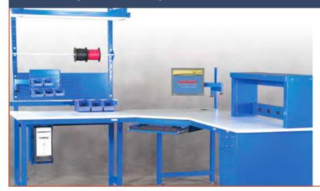
A corner workstation, utilizing components from the Series 5300 and 7000, exemplifies the versatility and flexibility of Workplace® Modular bench systems. This is an example of a multifunction workstation.
