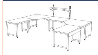
The functionality of the Series 5300 Quad work center line was the basis for the design of this spacious R&D area. Inner leg sections were specified as recessed legs to provide additional space. Cutouts with grommets are located at the rear of each corner to accommodate cabling.
