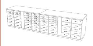
Eight individual Series 7000 cabinets form an in-line row. A wide selection of drawer configurations make it possible to choose the correct drawer arrangement for each application. The dimensions of this particular row is 30"Dx144"Lx36"H.
