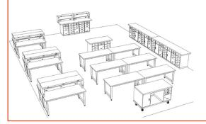
Series 4500 work tables are set back-to-back and end-toend; left row of tables are equipped with fixed riser shelves and wiretroughs. Series 7000 Banked Cabinet Stations and a Mobile Technician Station complete the lab.
