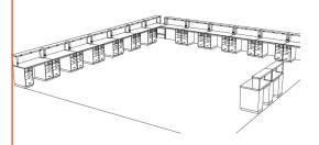
Eleven identical Series 7000 Cabinet-to-Cabinet Technician Stations frame two walls of this work environment. A third wall features an in-line Series 7000 Cabinet-to-Cabinet Station. All are equipped with fixed riser shelf assemblies outfitted with power. A space-saving corner unit unites the two longer rows together.
