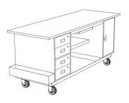
A combination of standard and customized components make up this mobile station. A customized "bottle holder" is mounted to the left end of the station and a center storage shelf and pull-out shelf are mounted between the two cabinets.
