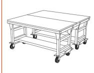
A spacious 60"Dx60"L Series 1000 Mobile table configuration is home to opthalmic instrumentation. The unit consists of customized Series 1000 framework which ties two individual units together.
