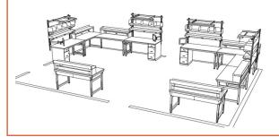
Overtable shelf storage was an important requirement for this application. Varying storage needs were met with a combination of fixed riser shelves, adjustable overtable shelves with back and end stops, and adjustable overtable divider shelves.
