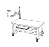
A flat screen articulating arm, keyboard tray, and Model N3114 drawer case accessorize a Series 4500 Mobile table for use in a DNA sequencing application.
