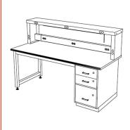
Hand-held radios are maintained and repaired on this Series 7000 Cabinet-to-Leg Technician Station. The 30"Dx72"Lx30"H unit has a plastic laminate top with post-formed front edge, and is equipped with a fixed riser shelf assembly and a 20-amp wiretrough.
