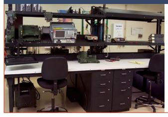
Back-to-back Series 7000 Technician Stations provide exceptional organization for an electronics shop application. Static protective laminate tops were selected for the 36"Dx72"L units. Overtable accessories include adjustable horizontal and sloping shelves, wiretroughs, and a flat-screen articulating arm with keyboard and tray monitor.
