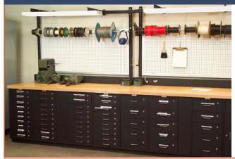
A 14' bank of eight cabinets provides considerable drawer storage for small parts and tools. The unit is topped with 1 3/4" thick maple tops for long-term durability. Overtable accessories include double Standard Uprights with pegboard panels, light suspension system with fixtures, 20-amp wiretroughs, and wirespool holders.
