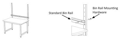
STANDARD BIN RAIL: Fasten Bin Rail to Solid Uprights using the mounting hardware in KIT-46A. If mounting to 3 Solid Uprights use KIT-46B.
