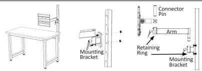
BIN ARTICULATING ARM: Fasten mounting bracket on Upright using hardware in KIT-56. Insert arm section into mounting bracket, fasten in place using the retaining ring. Use connector pin to mount bin attachment to arm section, fastening with retaining ring.
