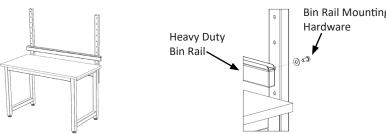
**HEAVY DUTY BIN RAIL**: Fasten Bin Rail to Solid Upight using the mounting hardware in KIT-52. If mounting to 3 Solid Uprights use KIT-52 plus KIT-53.
