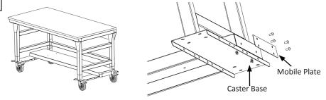
ON MOBILE CASTER BASE WITH PLATES: Position Shelf on lower crossmember of Leg Sections. Align holes on mobile plate with those on Shelf and on caster base, fasten using KIT-42.
