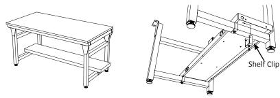
ON CROSSMEMBERS WITH BRACKETS: Set Shelf in desired position along lower crossbars of Leg Sections. Position shelf clips around lower crossbars with slits holding onto the return bend on the underside of the shelf. Tighten the set screw using the Hex Key found in 3016.
