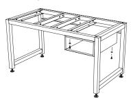
**ON A STANDARD\* WORKSTATION**: Align holes in top of Drawer Case or Pull-Out Shelf with snap-in nuts in Frame channel, fasten using KIT-09A.
