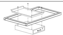
**ON A HEAVY-DUTY\*\* WORKSTATION**: Hang Bracket from Frame. Fasten Drawer Case or Pull-Out Shelf to the Bracket using KIT-09A.
