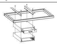
**TIERRING DRAWERS/PULL-OUT SHELF**: Align additional Drawer or Pull-Out Shelf Case with holes in mounted case, fasten down through upper case using KIT-09A.
