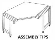
Assemble and fasten Corner Frames & Leg upside down. Flip Framework right-side up before attaching Wings or Tops.
