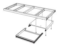
**ON A STANDARD\* WORKSTATION**: Mount Keyboard Tray, aligning pre-drilled holes in tray case with Frame. Fasten using KIT-17A. Return tray to case.
