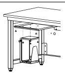
**ON A MOTORIZED BENCH**: Align mounting bracket to holes on the underside of Motorized Table, fasten with KIT-09A. Line up Caddy with threaded inserts in bracket and fasten with KIT-09A.
