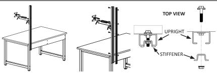
**SINGLE UPRIGHT STIFFENER**: *For mounting Articulating Arm on Single Upright* After arm has been mounted to Upright, place stiffener in rear channel of Upright, fasten using KIT-08B. Tighten to ensure stiffener is firmly set in Upright.
