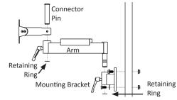
**FIXED HEIGHT ARTICULATING ARM**: Fasten mounting bracket on Upright using KIT-56. Insert arm section into mounting Bracket, fasten in place with retaining ring. Use connector pin to mount monitor attachment to arm section, fasten retaining ring.
