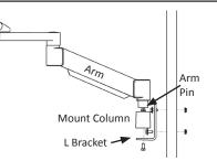
**FLOATING ARTICULATING ARM**: Fasten large "L" Bracket at desired location on Upright using KIT-103. Attach mount column to "L" Bracket using the 3/8-16 x 1/2" BHSCS and 3/8-16 Nut found in Flexmount hardware kit. Insert arm pin into mount column.
