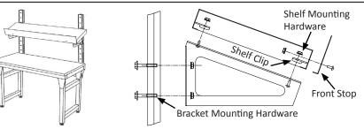
**SLOPED SHELF**: Fasten Front Stop to Shelf with KIT-16, lining up with holes in Shelf. Fasten Shelf Bracket to Solid Upight using the bracket mounting hardware in KIT-07C. Fasten the Shelf to Brackets using Shelf Mounting hardware.
