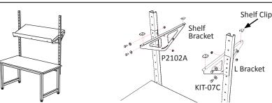
**CANTILEVERED**: Fasten Front Stop to Shelf with KIT-16, lining up with pre-drilled holes in Shelf. Fasten L Brackets to Solid Uprights using Bracket Mounting hardware in KIT-07C. Set Shelf Brackets to desire slope and fasten with P2102A flange nuts. Fasten Shelf to Brackets using Shelf Mounting hardware.
