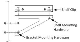
**FLAT SHELF**: Fasten Shelf Bracket to Solid Upright using bracket mounting hardware in KIT-07C. Fasten the Shelf to Brackets using shelf mounting hardware.
