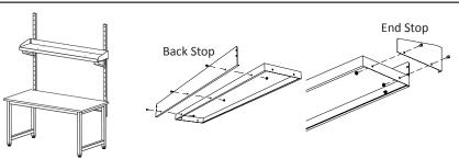
**BACK & END STOPS**: Align holes of Backstop with Shelf, fasten using KIT-15. Align holes of Endstops with Shelf edges, fasten using KIT-16. Fasten End Stops to Backstop using remaining KIT-15 hardware.
