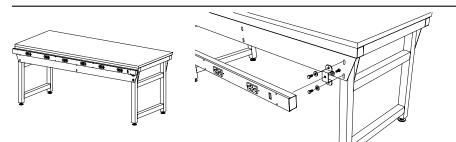
**REAR MOUNTING**: Mount 31131 Bracket to back of Powerstrip utilizing threaded inserts found in back of Powerstrip. Remove hardware from back of Swaybrace and set aside. Fasten Powerstrip/brackets to rear of Leg Sections using the previously removed hardware.
