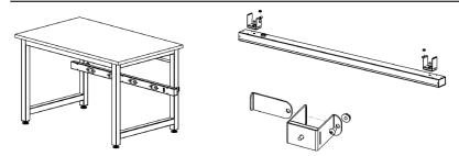
**MOUNTING ON LEG SECTIONS**: Mount leg bracket body to rear of Powerstrip using 1/4-20x1/2 RHMS. Hold Powerstrip/Bracket Assembly to Leg Sections (bracket body around Leg), slide rear plate through body and clamp to Leg using the 1/4-20 Flange Nut and 1/4-20x1/2 RHMS.
