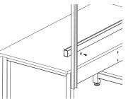
**MOUNTING TO UPRIGHTS**: Line up Powerstrip to desired location on Uprights, fasten with KIT-32A.
