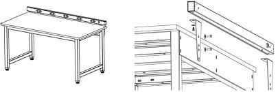
**MOUNTING WITH BRACKETS:** Align bracket lip to threaded inserts on bottom of Powerstrip, fasten 5/16-18 Flange Nut and Washer from KIT-23. Fasten Powerstrip/bracket assembly to Frame using remaining KIT-23 hardware.
