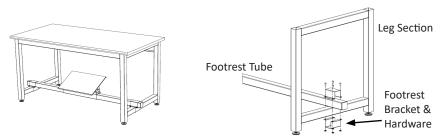
**TO LEG SECTIONS**: Slide the adjustable footrest onto the footrest tube. Mount the footrest tube to the lower crossbar (the tube can be mounted either above or below the crossbar) of leg sections using brackets and hardware from KIT-11.
